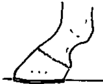
Fig. 16. Toe incorrectly dubbed off to fit shoe.
