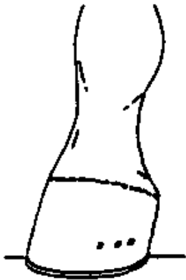
Fig. 24. Correct smooth, rectangular, tight clinches.
